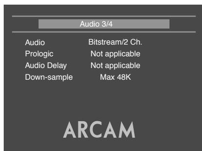
This section allows you to configure the type of analogue and digital audio outputs. In particular, the digital output type needs to be set correctly if you are using an external audio decoder, receiver or D-A converter.
